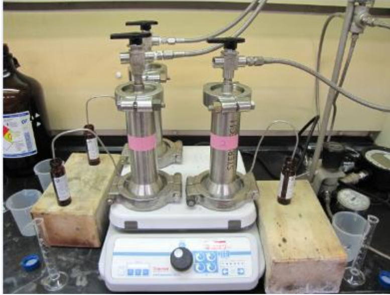
Figure 3-8: Membrane Bench Test Apparatus – As Tested
